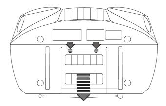
2.) Insert 8 UM-2 "**C**" size batteries into the battery compartment according to the polarity diagram engraved inside the compartment. If the batteries are inserted incorrectly the unit will not work.
